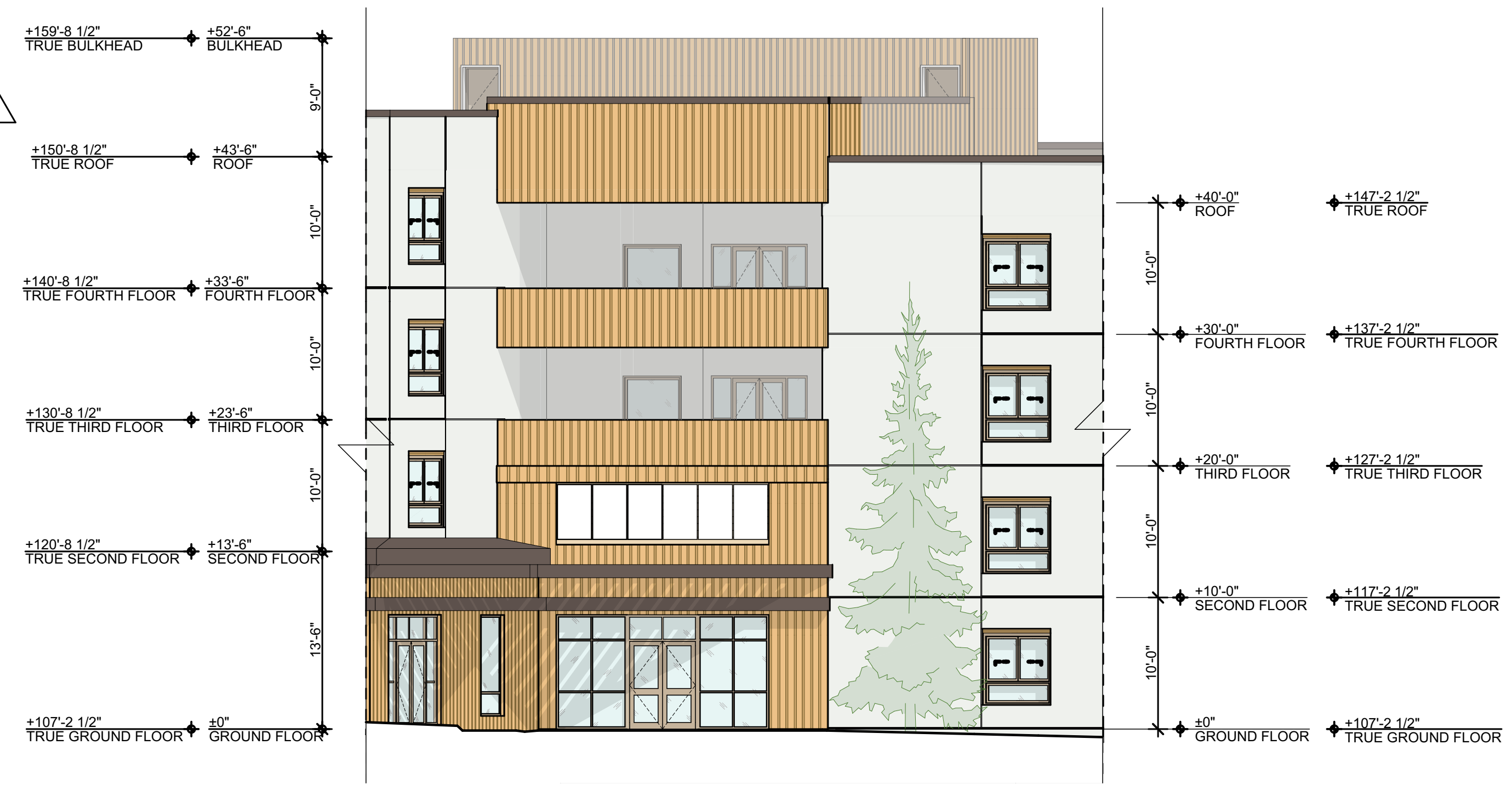
WING A - MAIN ENTRANCE ELEVATION ② SCALE: 1/8" = 1'-0"
