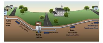
**Description:** The City owns and operates two lift stations to convey flow from low lying areas to high elevations where the flow continues by gravity to the wastewater treatment plant. Both pump stations have reached the end of their useful life and need to be rehabilitated.
